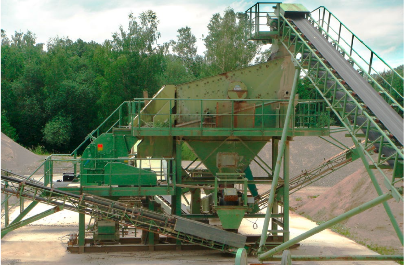
BHS Impact Mill of type PM 0806 for crushing concrete for recycling and for crushing oversized gravel. The Impact Mill is replacing a jaw crusher as part of a plant modernization process.
