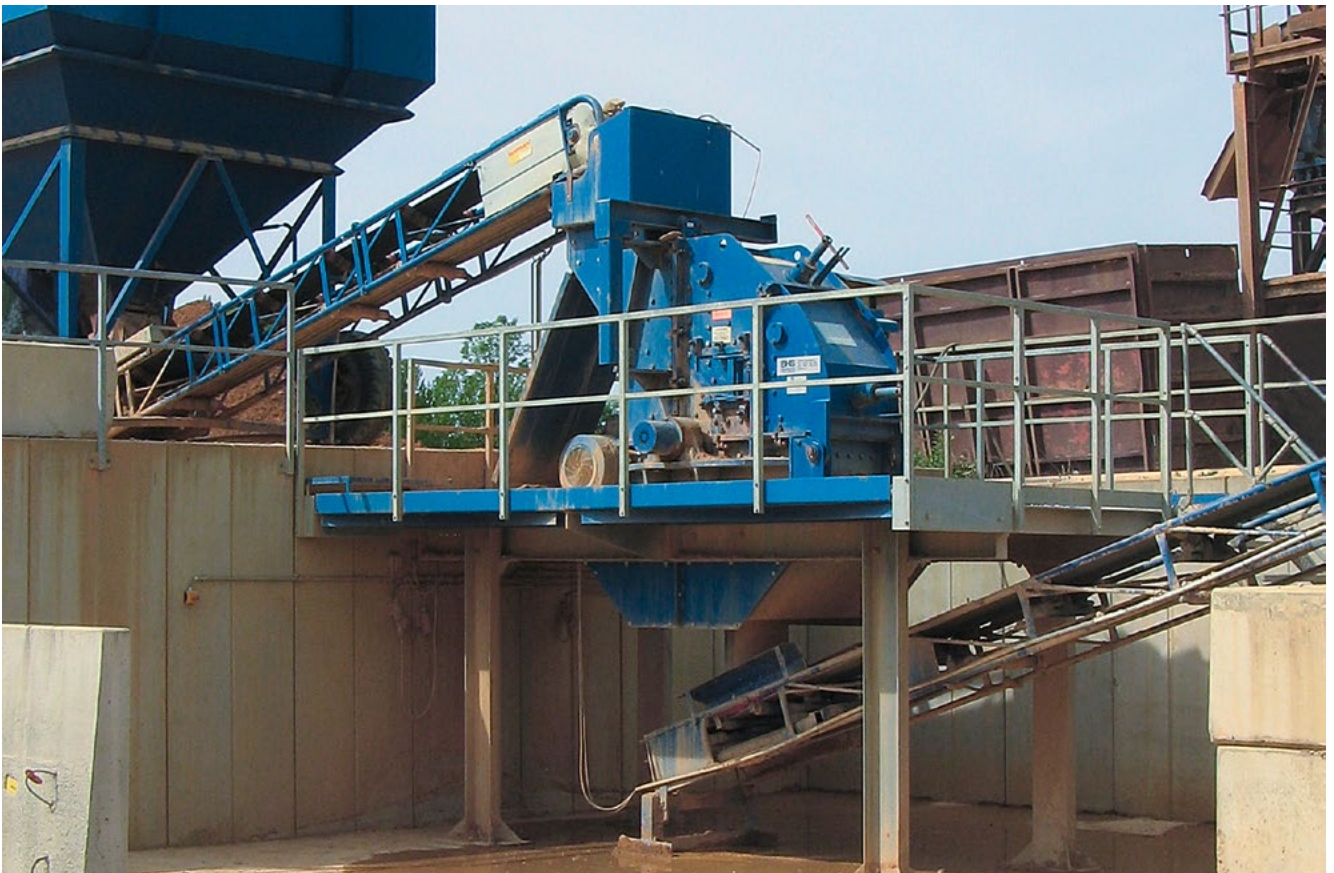
A BHS Impact Crusher of type PB 0806 is used for crushing oversized gravel (32 to 250 mm) to produce saleable chippings.
